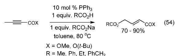
Scheme 5.5. Carboxylates as pronucleophiles in \gamma -addition to activated alkynes.
